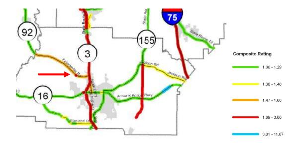
The capacity to illustrate alternatives is also shown. Instances where critical effects, such as a posted weight restriction of 30 to 39.9 percent of design load, can be identified (Eastern segment of GA-16), a more circuitous but efficient path can be observed. The decision to assign the corridor to the alternative, on a permanent basis, can be made by the collective stakeholder group.
