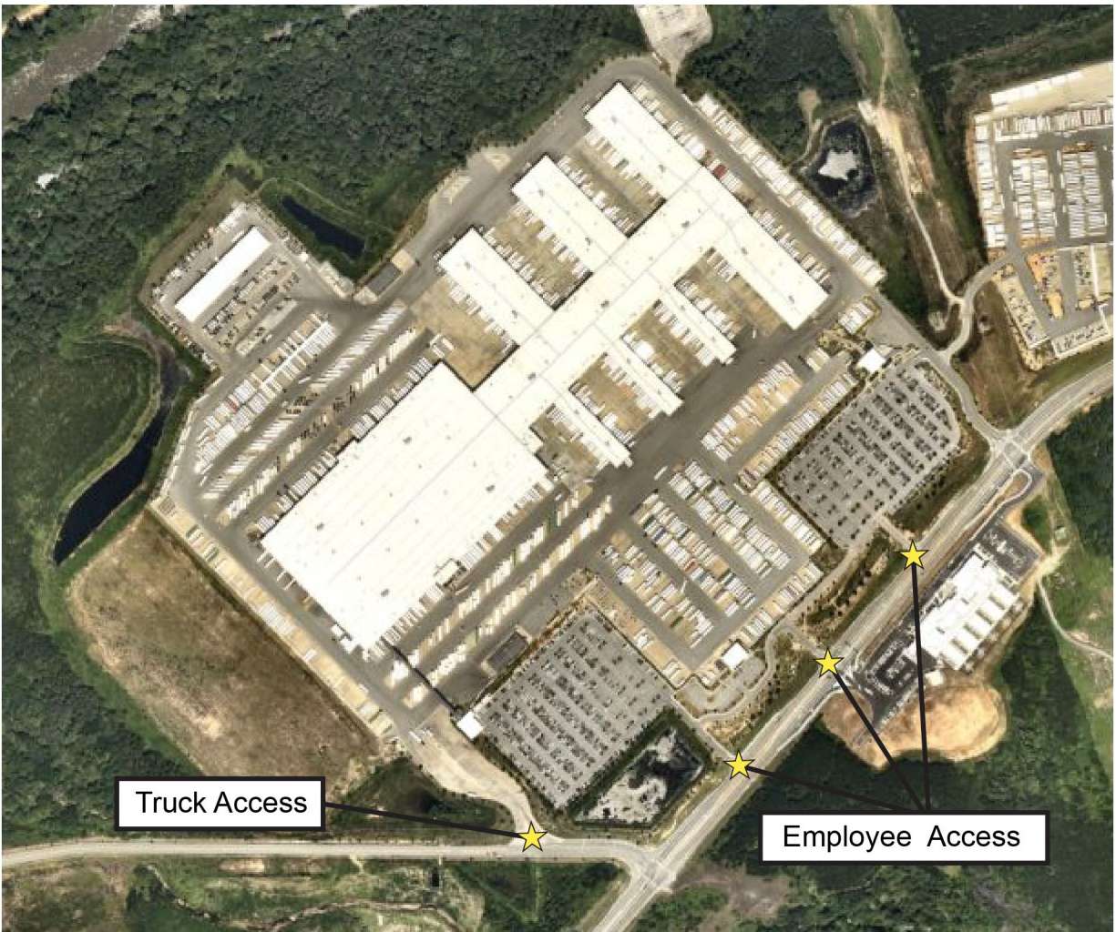
Figure 32: Separated Employee and Truck Access
