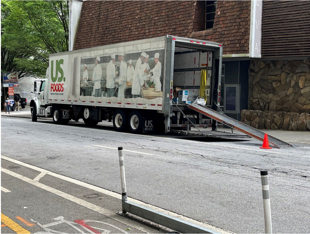
Figure 65: Truck Ramp Encroaching on Other Curb Spaces
