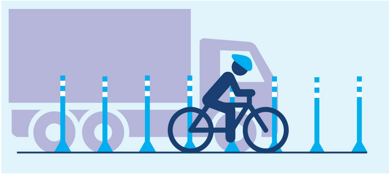
Figure 93: Illustration of a Vertical Buffer for Bike Lane
