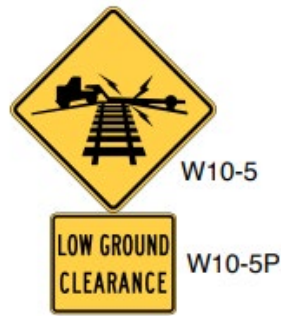
Figure 29: Low Railroad Clearance Warning Sign
