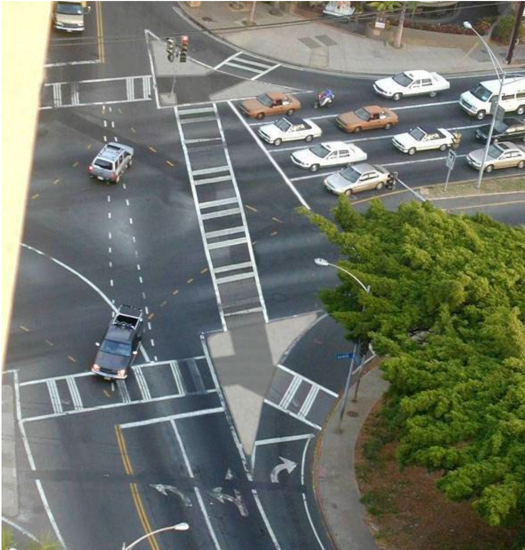
Figure 96: Channelized Right Turn Pedestrian Refuge Island
