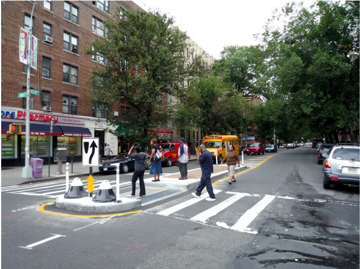
Figure 95: Pedestrian Refuge Area in Median at Intersection
