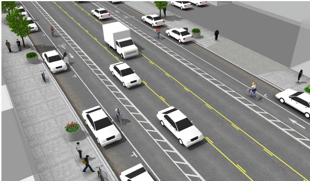
Figure 8: Buffered Parking Lane with Bike Lane
