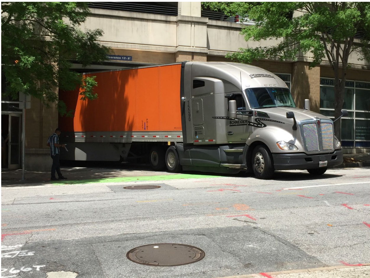
Figure 71: Truck in Loading Dock Spilling onto the Sidewalk and Street
