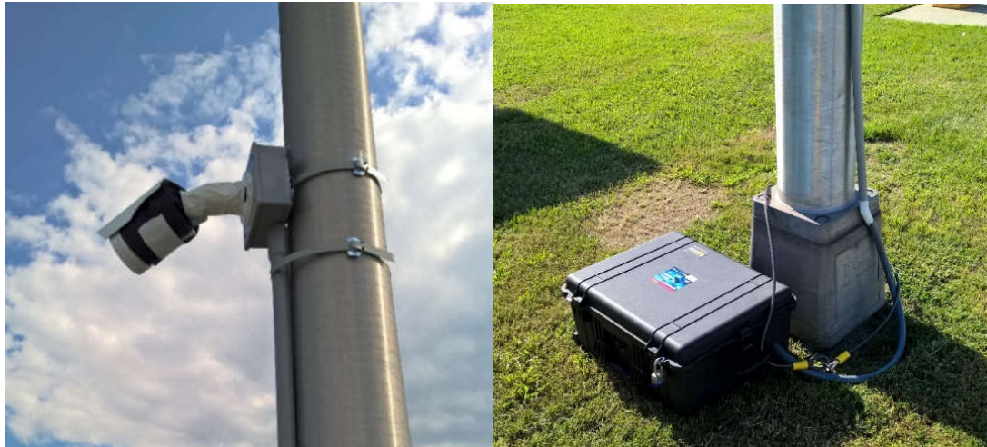
Figure 22. Installed camera, PVC conduit, and Pelican case
