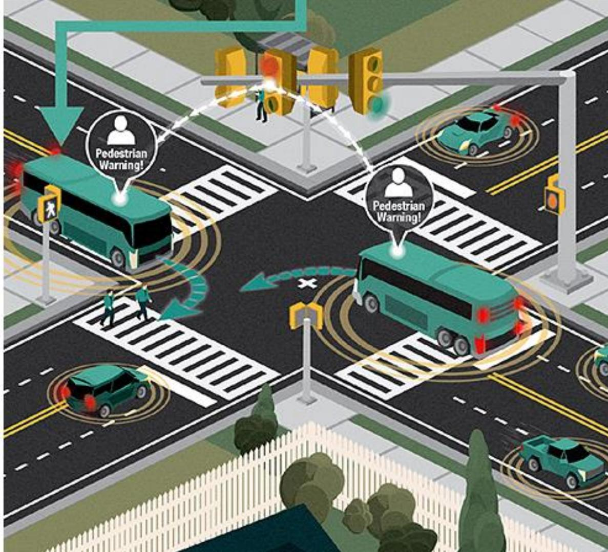
Warns drivers when a pedestrian is crossing the street as the vehicle is making a right or left turn.
